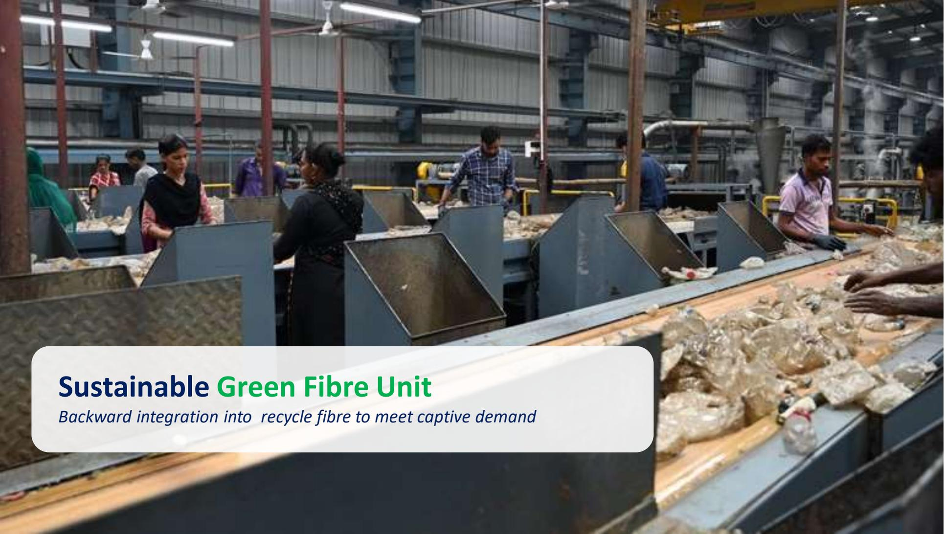
A wide-angle photograph of a large industrial facility, likely a recycling plant. In the foreground, a long conveyor belt is filled with clear plastic bottles and other debris. Several workers are positioned along the line, some wearing gloves and focused on sorting the waste. The background shows a complex network of metal structures, pipes, and overhead lighting, creating a busy and industrial atmosphere.
